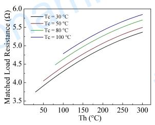
The chart for matched load resistance Vs T<sub>h</sub> under various T<sub>c</sub>
