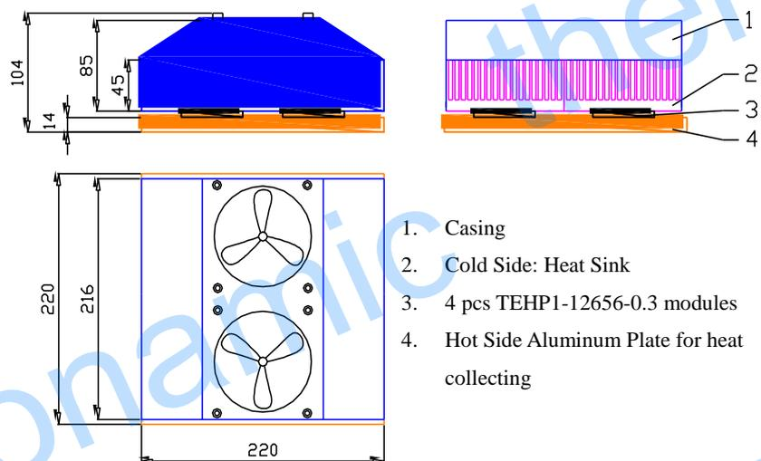
30 Watt Thermoelectric Generator Diagram
